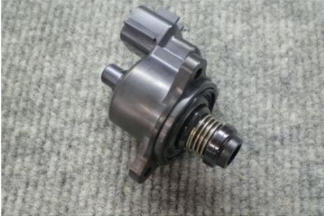
Idle valve stepper motor
