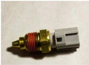
Coolant temperature sensor - single resistor type
