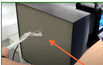
A smoke generator shows flow patterns around test objects
