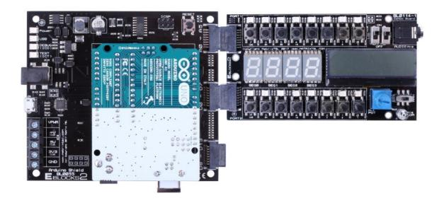
**Note:** Despite having two hardware port connections between the EB0114 Development board and the BL0055 Shield, the Arduino Uno can only provide 6 general purpose I/O connections on port C, (A0-A5).
