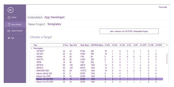
Select Arduino Uno R3 PDIP from the Free targets list. Click "New <Arduino..." button above
