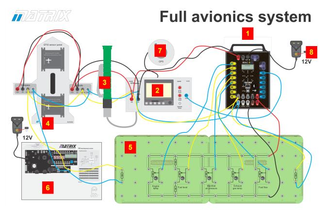
The image above shows all the parts of the EFIS system.
