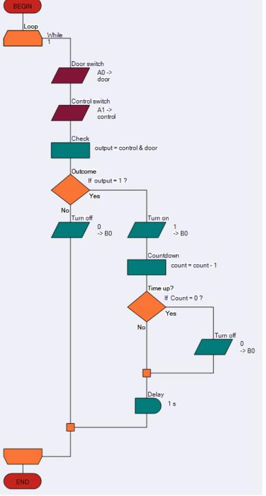
For Arduino the Ports need to be set to PORTC and PORTD (equivalent to A and B on the Combo board).
