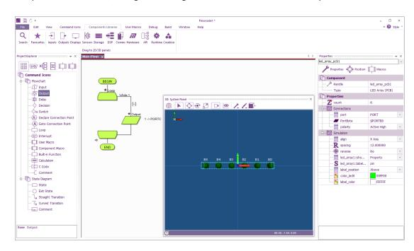
For example, the image above shows how **Flowcode First Program** (Page 42) would look to an Arduino user. Here, Arduino users are using **PORTC** instead of **PORTA**.
