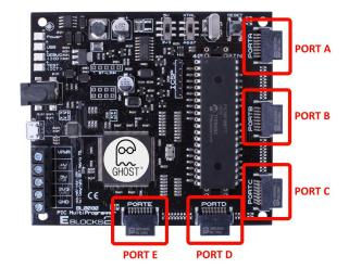
**Ports** - The PIC16F18877 PIC has five ports, labelled 'A' to 'E', connected to the rest of the microcontroller internals by an 8-bit bus system.
