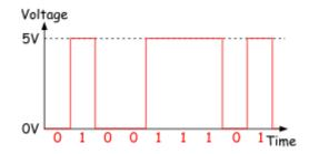
• The nine bit binary number represented by the signal is given under the waveform.
