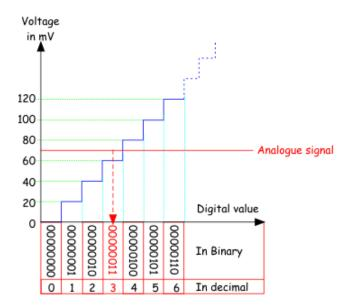
• In this example, the converter outputs '0000 0000' for any analogue signal up to 20mV, outputs '0000 0001' for analogue signals between 20 and 40mV, and so on.
