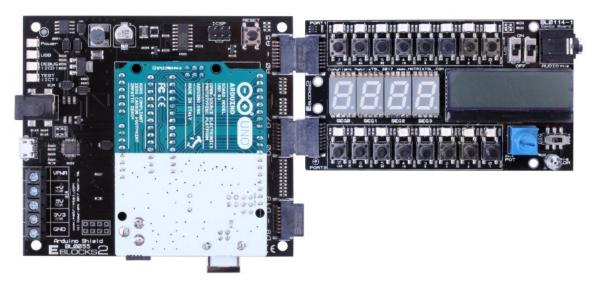
Eblocks2 uses the 'Click' boards for its SPI connections.
