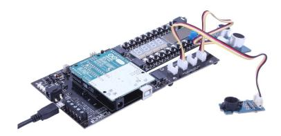
Upstream and downstream boards combined to form a full system, with the downstream boards plugging into the upstream 'intelligent' boards.
