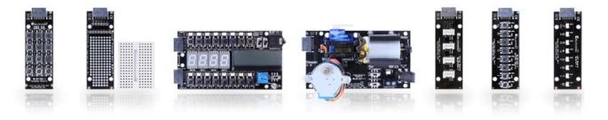
'Downstream' boards are controlled by an 'upstream' board, but information can flow into or out of them. Examples include LED boards, LCD boards, RS232 boards etc.
