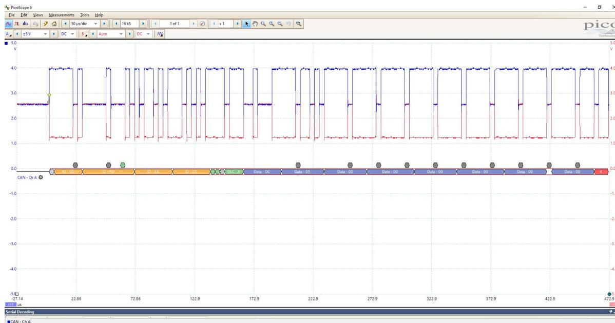
This system uses a CAN bus protocol called 'J1939'. Unfortunately, mainstream vehicle manufacturers do not publish details of how they have implemented the CAN bus protocol. In fact, most keep the details a close secret. The advantage of J1939 is that it is an open standard and there are many documents that supports its use.
