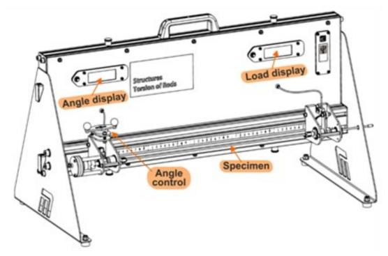
Turning the angle-control handle lowers the threaded bar and rotates the collet gripping the left-hand end of the rod. One full turn lowers it the bar by 1mm, causing the end of the rod to rotate by around 1.6°.
