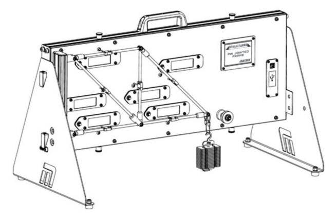
The framework is fixed at the left-hand end to an aluminium beam simulating a reaction wall. Each stainless steel member has at its mid-point a load cell linked to a LCD display. These displays measures the tension / compression force within each member. A negative reading on the load cell indicates a tension force in the member
