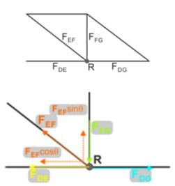
This time, force  $\mathbf{F}_{\mathbf{EF}}$  is resolved into horizontal and vertical components.
