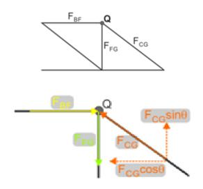
Force **F**<sub>CG</sub> is again resolved into horizontal and vertical components.
