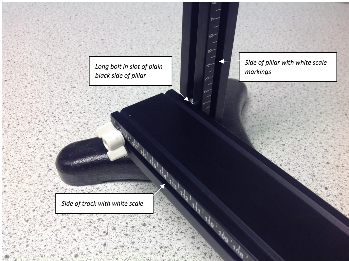
Setting up the pillar and track to avoid damage to the white scale markings
