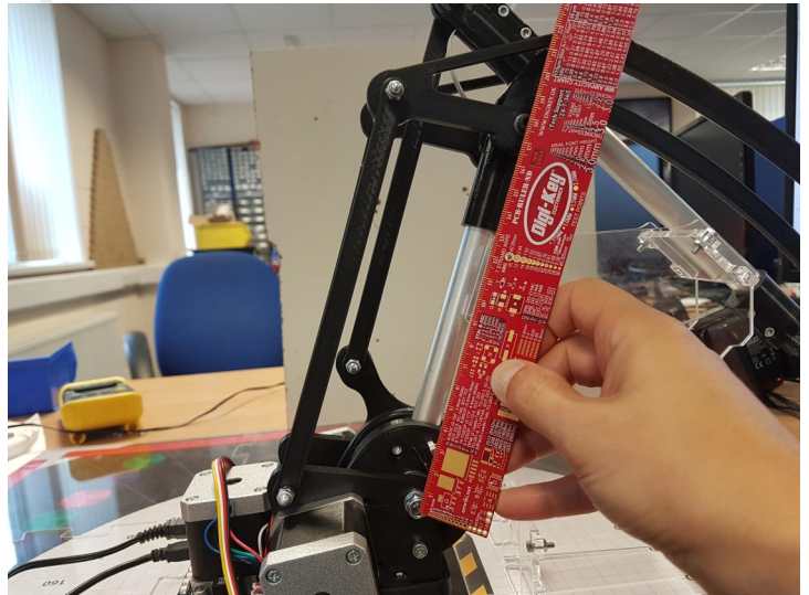
Measure and record the length of the shoulder, centre of main pivot to centre of bolt. The default is 176.0
