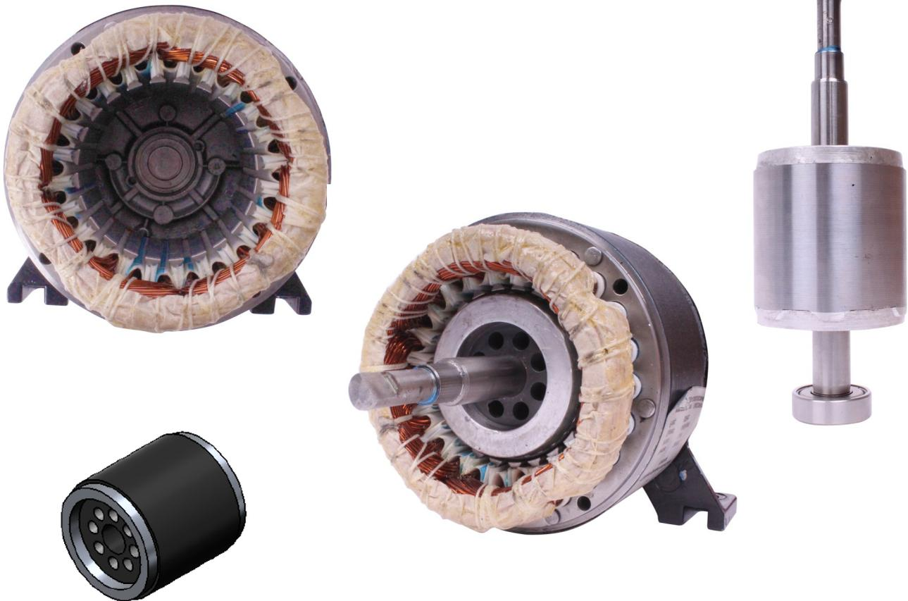
The three phase induction motor is the most common electrical machine in industry, where it used to drive pumps, fans, compressors and machine tools. Around 50% of the total industrial energy consumed in Europe is expended in motor drives of which an estimated 70-80% are induction motors.
