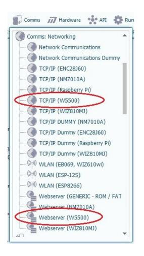
The TCP/IP and Webserver components can be found in the Comms section of the Component toolbar. These are identified by the W5500 device that is used on the ETH WIZ Click module.
