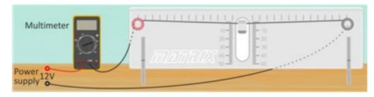
Linear expansivity is defined as the *fractional* change in length (increase in length / original length) occurring when the temperature rises by  $1^{\circ}$ C.
