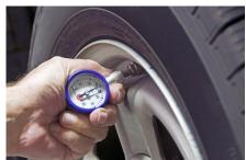
• Always check tyre pressures *before* you set off, not later! After driving for a while, the tyres heat up. The volume of air trapped in the tyre hardly changes but its pressure does.
