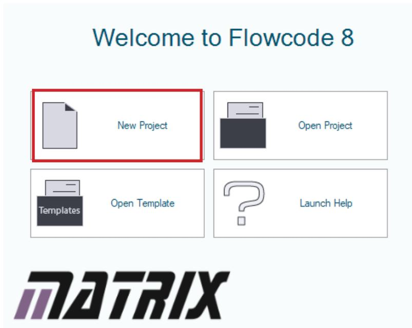
Once a new project is started, you need to select the correct microcontroller. As we are using an BL0011 board, with the default PIC16F18877 attached, we will need to ensure Flowcode has the corresponding chip selected. When using Matrix hardware, this has automatically been configured for the correct config properties and clock speed etc.
