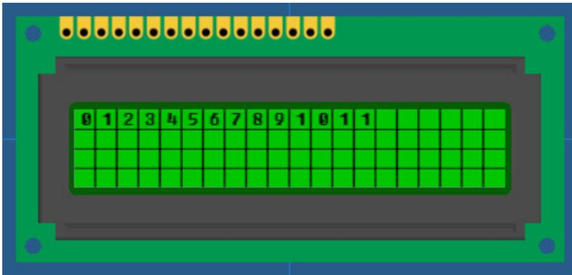
What we need to do is clear the LCD screen each time we write a new value. Luckily for us executing a clear screen routine also moves the cursor position back to (0,0). Add another component macro above the PrintNumber macro, and configure it to 'Clear'.
