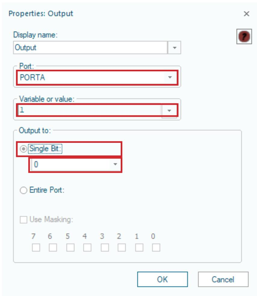
To make an LED flash we must turn it on and off. Place another output icon on your flowchart, below the original, and configure it as before. Although this time you should write a value of '0' instead to turn our LED off.
