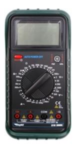
When using a multimeter to measure resistance, first remove the component from the circuit!
