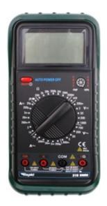
When using a multimeter to measure current, plug the probes into the 'A' and 'COM' sockets, or equivalents.
