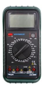
The picture shows one form of multimeter. It has a wide range of uses, which varies from model to model - but usually includes measuring AC and DC voltage and current.
