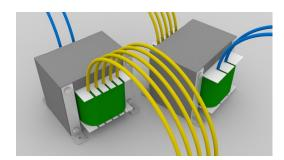
When the primary current is AC, the magnetic field varies. As the AC rises, falls and reverses, the magnetic field increases, falls and reverses in step with it. This moving magnetic field generates an alternating voltage in the secondary coil.
