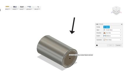
Enter the distance as a negative value to cut the part out. Confirm with enter and the area between polygon and circle will be removed.
