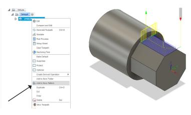
In this menu select Pattern Type: Circular pattern. Click on the rear cylinder. Before you confirm the box with ENTER, set the number of corners of your polygon under Number of Instances
