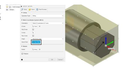
Switch to the tab Stock in the menu. Select the Mode: Fixed size cylinder. Click on the back part of your cylinder and enter the dimensions of the blank. In our example, the blank has the same size as the body we have created
