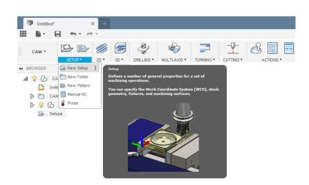
In this menu select the Operation Type: Milling. For Orientation set: Select Z-Axis/Plane & X-Axis. Click on the upper polygon surface. This aligns the Z axis. The blue arrow now points upward.
