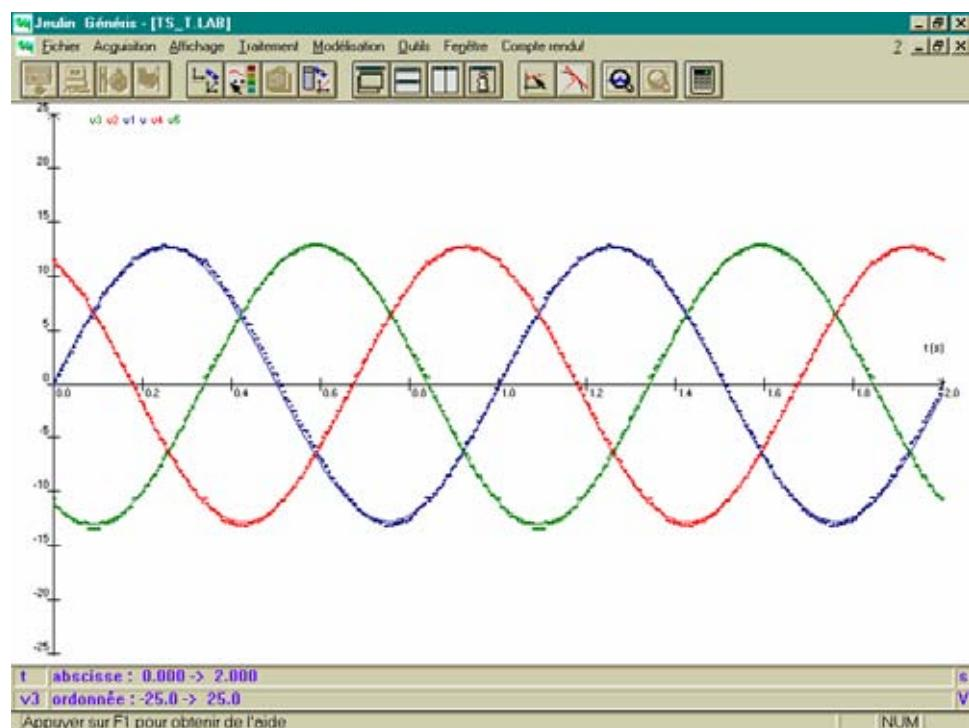
Check that  $v_1(t) + v_2(t) + v_3(t) = 0$  ( $\vec{V}_1 + \vec{V}_2 + \vec{V}_3 = \vec{0}$ ).
