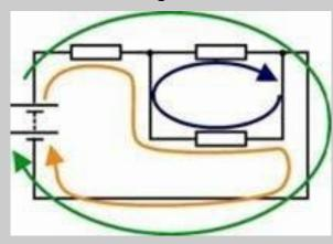
Around any loop in the circuit, the algebraic sum of voltages is zero.
