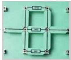
When resistors are connected in parallel, they offer different routes for the electric current. An easier route will pass a greater current.
