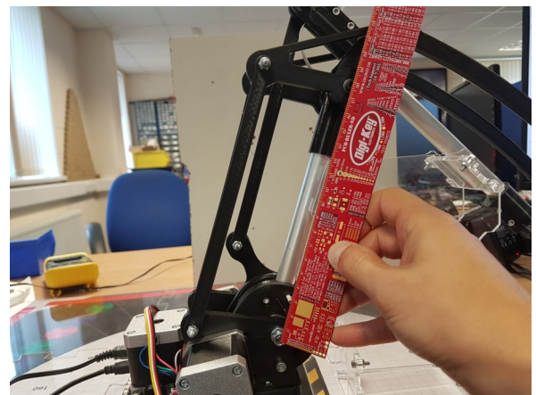
Measure and record the length of the shoulder - centre of main pivot to centre of bolt. The default is 176.0mm
