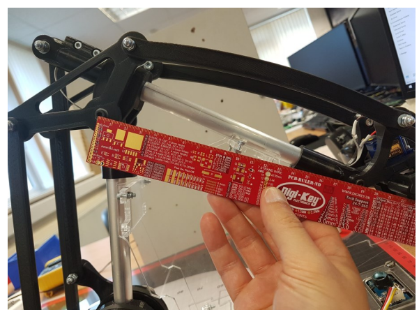
Measure and record the length of the elbow - centre of bolt to centre of bolt. The default is 189.0mm
