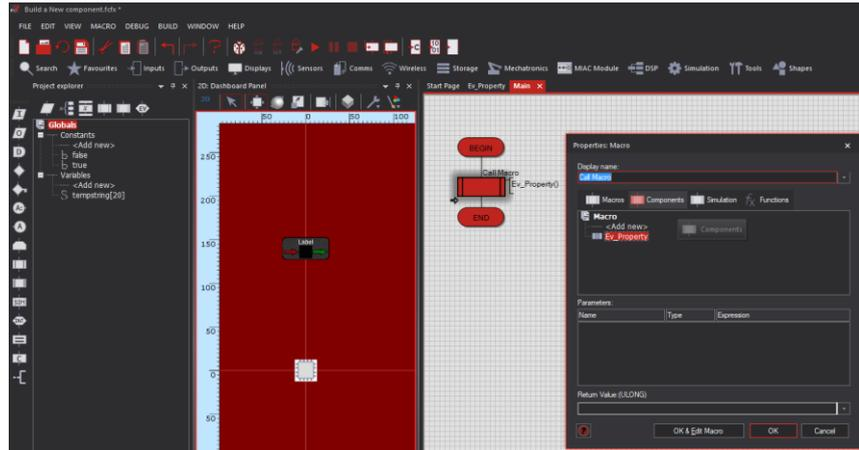
Now we need to put in those physical connections to the Chip. This has been made much easier with FC7. Simply click **Properties** and select add new. For the Cosmetic name **RX** and variable name **RX**. The Property **type**, select Single Digital Pin as shown.
