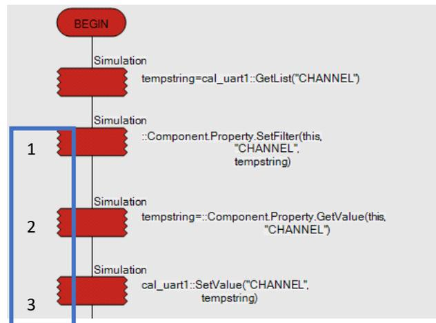
**1** - Under the **Functions TAB**– Select **Component – Property –** then **SetFilter** and for each of the following:
