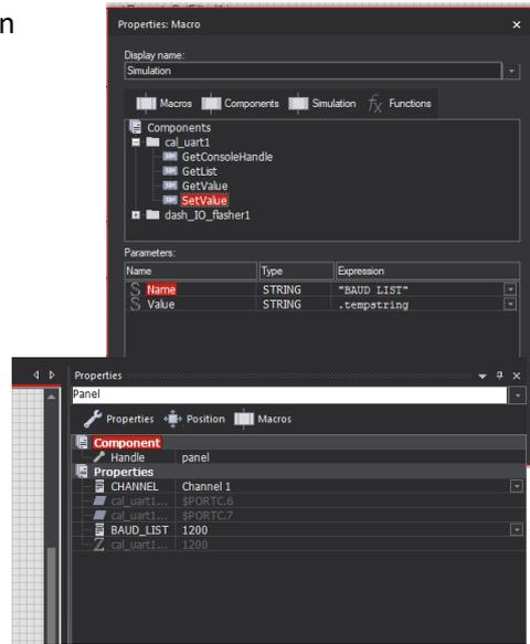
What we need to do now is make sure that whichever **Channel** is selected, the data is sent to the correct channel's **Pin connections**– either **Channel1** or **Software**. To do this we first place a channel switch into our **EV\_Property** Macro as shown below then send data to the correct pins for that channel. Channel 0 = Software           Channel 1 = Hardware
