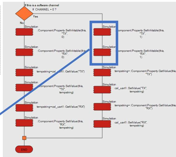
To set up the data flow, the top two simulation icons are copied across to the other side but the true/false is the opposite value as shown below.
