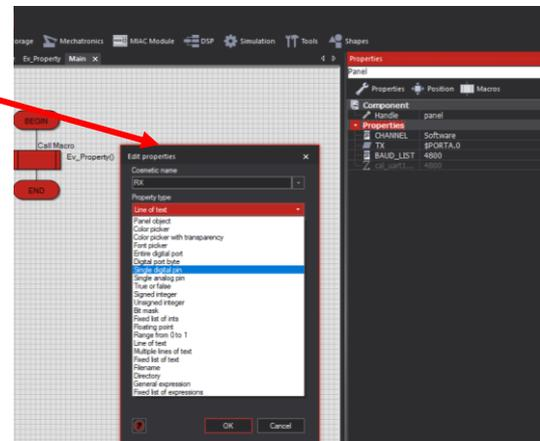
If you press **RUN**, then when you select your component you will see the options of **Channel 1** or **Software**. If you select the software option you will be able to select which pins of the chip are used for the RS232 port. Do that and then click onto the **Cal\_uart1** base component icon. Here you will see that the pins match what you have selected by your component. Remember though, you are controlling the connection of the base **CAL** from your component only!
