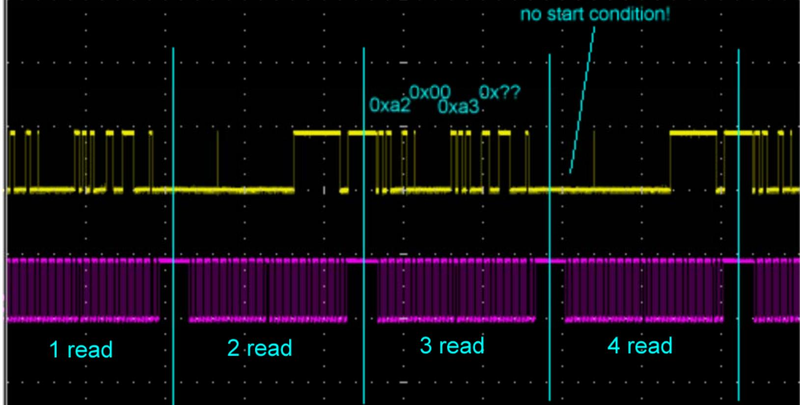
I2C in software mode on pins A7/B10 reads in a loop
