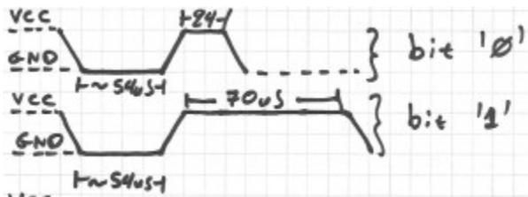
**End Of Frame:** At the end of packet DHT sends a  $\sim 54\mu\text{S}$  Low level, pulls the bus to High and goes to sleep mode.
