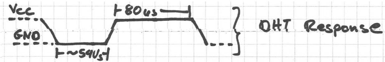
**3) Data Reading:** What will come after the response is the sensor data. The data will be packed in a packet of 5 segments of 8-bits each. Totally  $5 \times 8 = 40$ bits.
