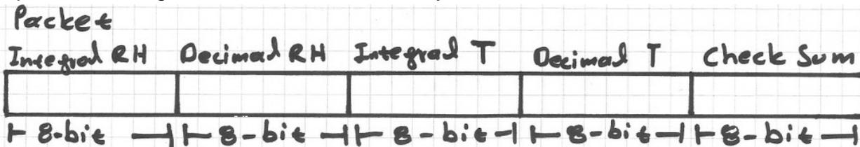
First two segments are Humidity read, integral & decimal. Following two are Temperature read in Celsius, integral & decimal and the last segment is the Check Sum which is the sum of the 4 first
