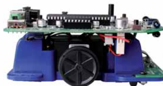
Plastic chassis with battery compartment, motors with gear boxes and 2 wheels
